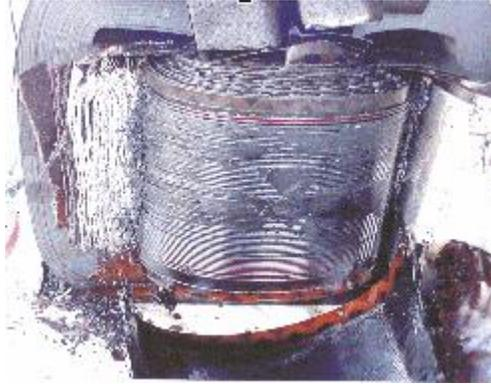
Figure 3: A Failed Distribution Transformer Due To A Heat Wave - Courtesy LADWP
